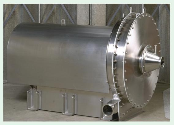
Halifax two-stage fan assembly, encased with a removable, polished, stainless steel shroud.
