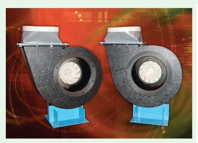
The new range is based on the existing fan range, covers a wide range of physical sizes and will offer duties up to 50,000m3/hr and pressures up to 5000Pa. Fan casings are fabricated from co-polymer black poly-propylene, embossed on the exterior surface to increase durability and scratch resistance, with the impeller removable from either the inlet or
